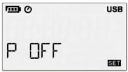
In the auto power-off setup page, press **UP** or **DOWN** button to enable or disable Power Off Function.
